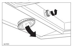
Turn the knurled screw counterclockwise. The halogen lamp will swivel down.
